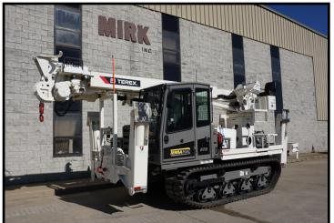
DIGGER DERRICK: **TEREX DISTRIBUTION DIGGER DERRICK MODEL: COMMANDER 4047** S.N. 2190568126 MOUNTED CENTER OVER REAR **OPERATOR'S RIDING SEAT** 18,660 LBS. MAX. CAPACITY **47' MAX. SHEAVE HEIGHT** SINGLE T-HANDLE CONTROL TRANSFERABLE POLE CLAWS TIP WINCH AND TOP CONTROLS PIN ON BUCKET W/ 300 LB. CAPACITY HYDRAULIC FIBERGLASS 3rd. STAGE 2 SPEED ; 12,000 FT. LB. DIGGER MOTOR **CONTINUOUS ROTATION 2 SETS RADIAL ARM OUTRIGGERS** HYDRAULIC TOOL CIRCUIT WITH RETRACT REEL **18" ROCK BULLET ROCK AUGER**
