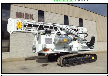
INNER KELLY WINCH: PULLMASTER M25 WITH CONTROLLED FREE FALL, 25,000 LBS. LINE PULL.
