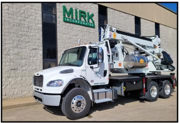
PRESSURE DIGGER SPECS. S.N. 23351 2023 WATSON MODEL 1100TM SHORT MAST JOHN DEERE 4045 DIESEL ENGINE (140 H.P.) FUNK MODEL 2000 TRANSMISSION 30 FEET OF DIGGING DEPTH ONLY 25 FT. OF MAST UP HEIGHT DRILL OUTPUT TORQUE UP TO 40,600 LBS. THREE ELEMENT KELLY BAR. 7" - 5" - 3 1/2" 4" KELLY STUB CROWD FORCE— 21,300 LBS. 8500 LB. SERVICE WINCH ROTATING AND SLIDING BASE (24" OF TRAVEL) OUTRIGGERS: OUT & DOWN FRONT, STRAIGHT DOWN REARS
