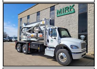
BODY SPECIFICATIONS: ALL STEEL CONSTRUCTION FLATBED FRONT DECK EXTENSION FOR AUGER STORAGE (2) UNDERDECK STORAGE BOXES H.D. PINTLE STYLE HITCH SAFETY CHAIN EYES 7 PRONG TRAILER PLUG AXLE WEIGHTS EMPTY: FRONT AXLE: 10,380 LBS REAR AXLES: 31,200 LBS TOTAL: 41,580 LBS <u>MIRK #</u> 835J
