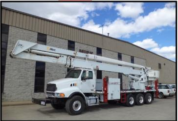
MATERIAL HANDLING AERIAL DEVICE: ALTEC MODEL HL-125 S.N. 080510147 120' TO BOTTOM OF BUCKET 125' OF WORKING HEIGHT MAXIMUM SIDE REACH 45.5 FT. LOWER BOOM TELESCOPIC EXTENSION 40 FT. FIBERGLASS 2 MAN BUCKET WITH HYD. ROTATOR MAX. BKT. CAP. 800 LB. MAX. JIB CAP. 1500 LB. PLATFORM & JIB CAP. COMBINED 2100 LB. HYD. JIB AND WINCH WITH HYD. EXTEND & ARTIC. MAXIMUM DIELECTRIC RATING 500 KV CAT-A CONTINUOUS ROTATION 2 HYDRAULIC TOOL CIRCUITS @ BUCKET 4 RADIAL ARM STYLE OUTRIGGERS
