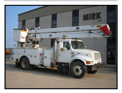
BODY: FULL LINE BODY MASTER ROD LOCKING SYSTEM HOT STICK COMPARTMENT FIBERGLASS TILT FRONT END W/ SERVICE ACCESS CURBSIDE ENTRY WAY PINTLE HITCH SAFETY CHAIN EYES 7-PRONG TRAILER PLUG TAIL SHELF WITH TUNNEL STORAGE HYD. TOOL CIRCUIT AT BUCKET & GROUND LEVEL
