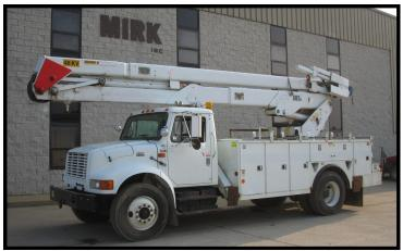
AERIAL DEVICE: HOLAN MATERIAL HANDLER MODEL # 80-5B-55-3 55' HEIGHT TO BOTTOM OF BUCKET 60' WORKING HEIGHT SINGLE HANDLE UPPER CTR 47' 9" MAXIMUM REACH FROM CENTERLINE TWO MAN HYDRAULIC ARTICULATED BASKET 700 LB. BUCKET CAPACITY 1500 LB. HYD. TILT JIB CAPACITY; HYD. EXTEND CONTINUOUS ROTATION ; 360 DEGREES LOWER OVER RIDE CONTROLS LOWER BOOM INSERT ;105 DEGREES ARTIC. INSULATED UPPER BOOM; OVERCENTER HYDRAULIC TOOL CIRCUIT AT BASKET FRONT AND REAR "A" FRAME OUTRIGGERS
