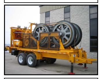
DIMENSIONAL DATA: LENGTH OVERALL: 315" (26'6") WIDTH OVERALL: 108" (9') WITH OUTSIDE TIRES ON WITHOUT OUTSIDE TIRES: 96" (8'6") HEIGHT OVERALL: 150" WITH ROLLERS ON WITHOUT ROLLERS: 138" (11'6") TOTAL WEIGHT: APPROX. 34,000 LBS. MANUAL PIN IN PLACE FRONT OUTRIGGERS
