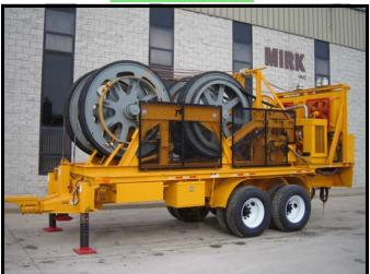
PERFORMANCE CHARACTERISTICS: BASED ON OPERATION WITH A SUITABLE LET-OFF STAND. TWO SUB CONDUCTORS 5,000 LBS. AT 7.0 M.P.H. 7,500 LBS. AT 5.3 M.P.H. 10,000 LBS. AT 3.5 M.P.H. 15,000 LBS. AT 2.5 M.P.H. SINGLE CONDUCTOR WITH COUPLING OF MODULES. 25,000 LBS. AT 2.5 M.P.H.
