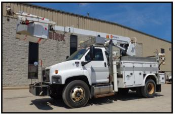
CABLE PLACER AERIAL DEVICE: POSI+ MODEL 800-40-025 S.N. 08-11-683-2533 NON-INSULATED ARTICULATING & TELESCOPIC STEEL BOOMS MAX. PLATFORM HEIGHT 35' MAX. WORKING HEIGHT 40' MAX. SIDE REACH 29.3' SINGLE HANDLE PROPORTIONAL CONTROL LOWER OVERRIDE CONTROLS 30" X 30" BASKET (350 LB. CAP. ) 120V AC CIRCUIT AT BOOM TIP WITH OUTLETS AT PLATFORM DUAL BOOM TIP REC. AND PULLING EYE ASSY. 370 DEGREES OF NON-CONTINUOUS ROTATION 2-WAY VOICE COMM. SYSTEM (PLATFORM/CAB)
