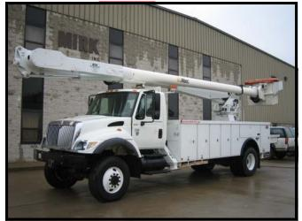
TRUCK MOUNTED AERIAL DEVICE: ALTEC MODEL # AM-900 67' TO BOTTOM OF BUCKET 72' OF WORKING HEIGHT 2 MAN END HUNG BUCKET (700 LB. CAPACITY) INSULATED UPPER BOOM (46 K.V. AND BELOW) LOWER BOOM INSERT (2) HYDRAULIC TOOL CIRCUITS AT BUCKET SINGLE HANDLE UPPER CONTROL CONTINUOUS ROTATION (4) "A" FRAME HYDRAULIC OUTRIGGERS EMERGENCY POWER STOP/ START LOWER OVER-RIDE CONTROLS
