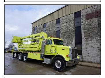
BODY 29' TREADPLATE FLATBED UNDERBODY BOXES 2 2 **DECK MOUNTED TOOL BOXES PINTLE HITCH 7-PRONG TRAILER PLUG** SPLASH APRONS 40' OVERALL LENGTH 12'10" STOWED HEIGHT AXLE WEIGHTS: EMPTY STEER AXLE: LBS. **DRIVES:** LBS. AIR TAG @ 80 PSI: LBS. **TOTAL WEIGHT:** LBS.
