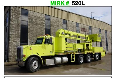
BRIDGE INSPECTOR: ASPEN AERIALS UNIT UB50 (REACH ALL) BRIDGE INSPECTION UNIT MODEL # 4045 BASKET CONTROLS / LOWER OVERRIDE CONTROLS TELESCOPIC 3RD BOOM HYDRAULICALLY ACTIVATED 4TH BOOM 40" X 60" X 42" 2 MAN ALUMINUM BASKET 600 LBS. BASKET CAPACITY TWO ROTATING TURRETS (T-1 + T-2) INTERCOM SYSTEM (BASKET TO CAB) UNIT POWER TAKE OFF FROM (TRUCK) 51' 9"HORIZONTAL REACH BACK UNDER THE BRIDGE 63' DOWN REACH VERTICAL FROM BRIDGE DECK
