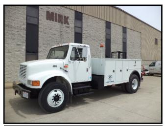
UNDERGROUND WINCH: ADAMS CD-28 20,000 LB. BED WINCH WITH LEVELWIND AND EXT. SHAFT MAX. 2,000' OF 1/2" WIRE ROPE ON DRUM ALL ANGLE SHEAVE MTD. AT REAR HYDRAULIC TOOL CIRCUIT WINCH HAS 3 SPEED CONTROL AND DRUM FREE-WHEEL OPERATORS PROTECTION CAGE RIGHT REAR ELECTRONINC THROTTLE CONTROL
