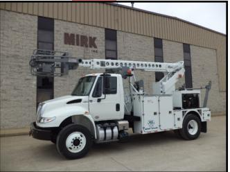
AERIAL STRINGING DEVICE: **RE-MOUNTED TELSTA T-40C PRO SERIES 40' WORKING HEIGHT** HYDRAULIC BASKET LEVELING **500 LBS. BASKET CAPACITY** 2,000 LBS. BOOM LIFTING EYE **DIESEL ONAN GEN-SET** SINGLE HANDLE JOYSTICK UPPER CONTROL LOWER OVERRIDE CONTROLS **START/STOP** @ BASKET TOW LINE CONTROL @ BASKET EMERGENCY LOWERING **HYD. REEL CARRIER WITH POWER WIND 110V PLUMBED TO THE BASKET INTERCOM SYSTEM TO BASKET** ALL STRINGING FAIRLEADS AND ROLLERS
