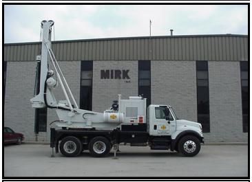
BODY SPECIFICATIONS: ALL STEEL CONSTRUCTION FLATBED FRONT DECK EXTENSION FOR AUGER STORAGE (2) 18" X 48" UNDERDECK STORAGE BOXES H.D. PINTLE STYLE HITCH SAFETY CHAIN EYES 7 PRONG TRAILER PLUG FRONT AXLE: 10,400 LB. REAR AXLES: 31640 LB. TOTAL: 42040 LB. EMPTY
