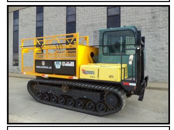
(1) 18' X 72" EXPANDED METAL STORAGE BIN SWING OPEN REAR BAR FOR REELS OF ROPE OR WIRE STORAGE CHAIN HOIST STORAGE BAR MTD RT. REAR TIE DOWN EYES LOCATED THRU OUT BED
