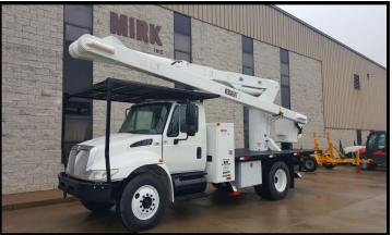
AERIAL DEVICE: VERSALIFT VO- 255 LOWSTOW 55' PLATFORM HEIGHT 60' WORKING HEIGHT 46' HORIZONTAL SIDE REACH 270 DEGREE INSULATED UPPER BOOM CATEGORY C 46KV AND BELOW 125 DEGREE LOWER BOOM WITH INSERT HYDRAULIC TOOL CIRCUIT AT BUCKET SINGLE HANDLE UPPER CONTROLS 360 DEGREE CONTINUOUS ROTATION 4 HYDRAULIC OUTRIGGERS 350 LB. BUCKET CAPACITY
