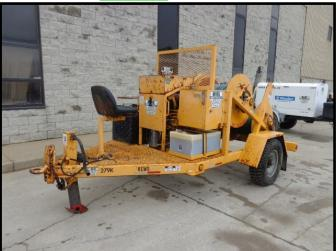
LINE PULL MAX. 19,800 IN. LBS.EACH DRUM DRUM DIMENSIONS: INSIDE WIDTH: 23" OUTSIDE DIAM: 33" CORE DIAM: 10 3/4" DRUM CAPACITY: 6000' OF 1/2" ROPE 4 ROPE COLORS: RED, GREEN, BLUE, YELLOW
