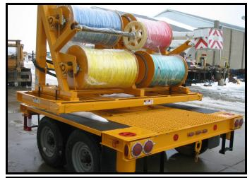
PERFORMANCE SPECS. BASED ON 15 G.P.M. @ 2000 PSI. RATED LINE PULL: 1650 LBS. EMPTY DRUM 875 LBS. FULL DRUM MAXIMUM LINE PULL: 2000 LBS. EMPTY DRUM 1000 LBS. FULL DRUM BASED ON 3000 PSI. INTERMITTENT ONLY LINE SPEED: 0-270 F.P.M. EMPTY DRUM 0-540 F.P.M. FULL DRUM AVERAGE LINE SPEED: 396 F.P.M. 5,280 ' OF 3/8" ROPE PER DRUM 4 COLORS RED, WHITE, BLUE, GREEN
