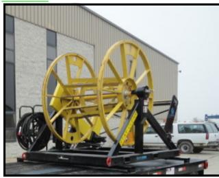
MAXIMUM REEL CAPACITY: 45" MAXIMUM WIDTH 90" MAXIMUM DIAMETER 20,000 LBS. MAX. WEIGHT TAG READS S.N. AF301 MODEL: 21032655 MFG. DATE: 4-25-2011
