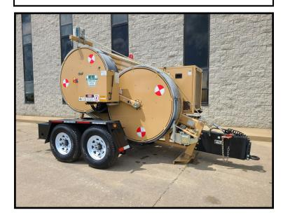
**NEGATIVE SELF ACTING HYDRAULIC BRAKE HYDRAULIC DYNAMOMETER** HYDRAULIC OIL COOLING SYSTEM **GEAR BOX WITH 2 OPERATING POSITIONS & 1 NEUTRAL POSITION** LOW PULL/TENSION POSITION (350-1800 LBS.) HIGH PULL/TENSION POSITION (1350-10,100 LBS.) HYDRAULIC ACTUATED FRONT PLOW
