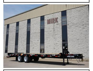
DIMENSIONAL DATA: OVERALL WIDTH: 102" OVERALL LENGTH: 447.6" OVERALL HEIGHT: 35" TALL RAMPS: 6' X 20" SPRINGS 49" SPREAD GVWR: 53,90 ENTIRE UNIT PAINTED BLACK WITH D.O.T. REFLECTIVE TAPE CARGO DATA: CARGO AREA—24' X 8.5' BEAVERTAIL: 6' X 8.5' BUIILT IN STORAGE BOX IN A-FRAME AREA OF HITCH
