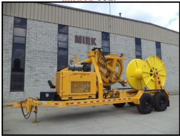
**ELASTOMER BULLWHEEL SEGMENTS** THE MACHINE DESIGN INCORPORATES A PIVOTING **BULLWHEEL WHICH AUTOMATICALLY ALIGNS THE BULLWHEEL WITH THE POINT ON THE REEL FROM** WHICH THE CONDUCTOR IS BEING PAYED OFF. DURING THE PULLING MODE THE OPERATOR CONTROLS THE **BULLWHEEL MOVEMENT TO LEVELWIND THE PULLED CABLE ONTO THE STORAGE REEL**
