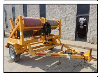
DIMENSIONS: LENGTH: 12 FT. 6 IN. WIDTH: 8 FT. 3 IN. HEIGHT: 6 FT. 6 IN. WEIGHT: (LESS ROPE) 2100 LBS. GVWR: 10,000 LBS. MOUNTED ON SINGLE TRAILER FOR TRANSPORT REAR PULL ONLY WHILE MTD. ADJUSTABLE PINTLE STYLE HITCH SAFETY CHAINS 7 PRONG TRAILER PLUG
