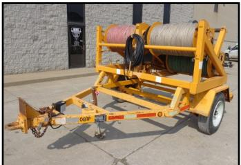
PERFORMANCE SPECS. BASED ON 15 G.P.M. @ 2000 PSI. RATED LINE PULL: 1650 LBS. EMPTY DRUM 875 LBS. FULL DRUM MAXIMUM LINE PULL: 2000 LBS. EMPTY DRUM 1000 LBS. FULL DRUM BASED ON 3000 PSI. INTERMITTENT ONLY LINE SPEED: 0 –270 F.P.M. EMPTY DRUM 0—540 F.P.M. FULL DRUM AVERAGE LINE SPEED: 396 F.P.M. 5,280 ' OF 3/8" ROPE PER DRUM 4 COLORS RED, WHITE, BLUE, GREEN
