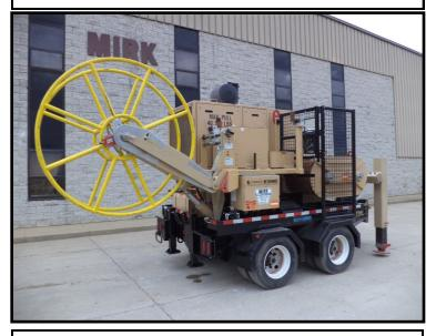
HYD. EXTERNAL DRUM SAFETY CLAMP TO HOLD CONDUCTOR AGAINST PULLING DRUM OPTIONAL ELECTRONICPULL AND SPEED RECORDER ADJUSTABLE SIDE TO SIDE FAIRLEAD ROLLER FOR PULLING LINE. AIR BRAKES APPROX. TOTAL WEIGHT: 19,000 LBS.
