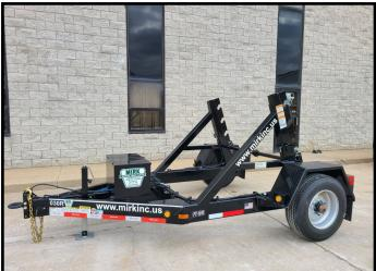
MAXIMUM REEL CAPACITIES: MAX. REEL WIDTH: 60" (59" IF BELOW STUBS) MAX. REEL DIAM: 120" MAX. WEIGHT: 9,400 LBS. 2 1/4" SOLID ARBOR BAR 12 VOLT D.C. BATTERY WITH CHARGING SYSTEM CHARGED THRU TRAILER PLUG FROM TOW VEHI-CLE.
