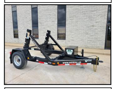
BODY DIMENSIONAL DATA: OVERALL LENGTH: 144" OVERALL WIDTH: 102" OVERALL HEIGHT: 76" PAINTED: BLACK POWDER COAT EMPTY WEIGHT: 2,100 LBS.
