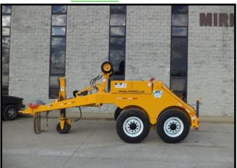
HYD. SELF LOADING REEL TRAILER GASOLINE 2 CYLINDER ENGINE HYDROSTATIC DRIVE SYSTEM 3" REEL MANDREL (ARBOR BAR) REAR MANUAL STABILIZER JACKS RIGHT FRONT CONTROLS LOCATION DRIVE WHEELS ARE EASILY ADJUSTED FOR REEL WIDTH BY MANUALLY SLIDING HYDRAULIC RESERVOIR BUILT INTO THE TRAILER MAIN FRAME. 2 BUILT IN STORAGE COMPARTMENTS ON
